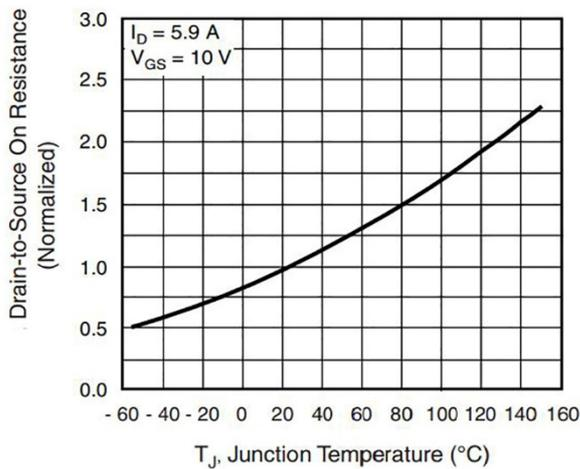
**Figure 7.8** Variation of ON-resistance with temperature IRF630
