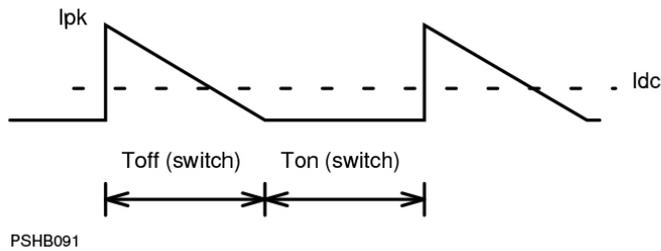
**Figure 7.14 Flyback output diode current- discontinuous mode**
