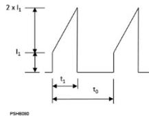
**Figure 7.4 Recommended flyback waveform**
