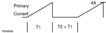
**Figure 7.7** Flyback primary current on the edge of CCM/DCM at 50% duty cycle
