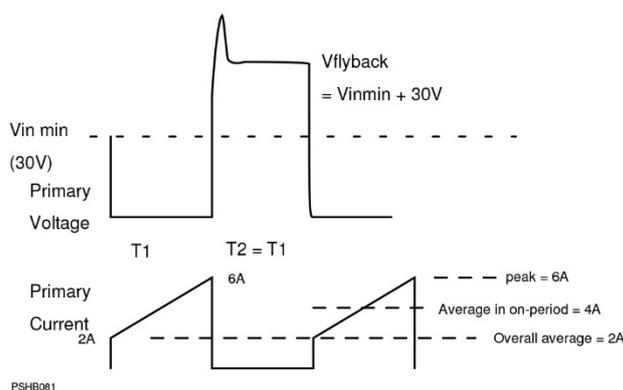
**Figure 7.5 Flyback primary voltage and current waveforms - 50% duty cycle and Vin minimum**
