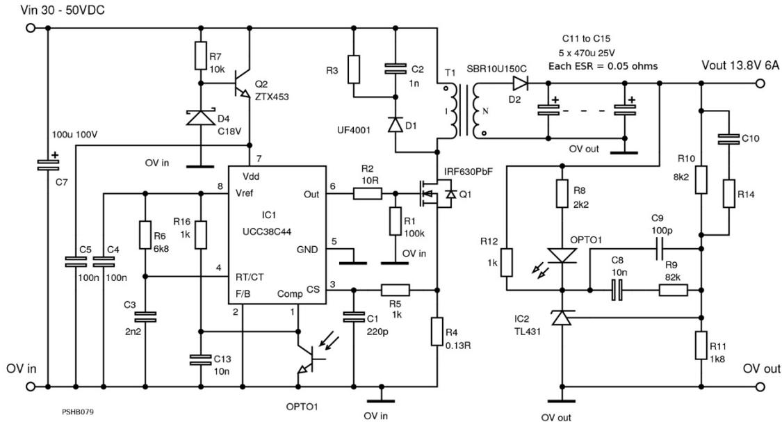
**Figure 7.10** Example isolated flyback circuit
