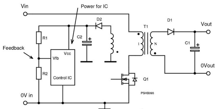
**Figure 7.16** Primary referenced winding provides semi-regulation
