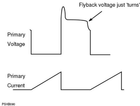
**Figure 7.13 Flyback critical conduction mode waveforms**
