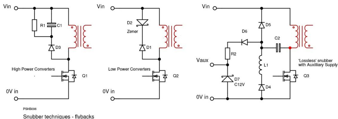
**Figure 7.9** Snubber techniques for flyback circuits
