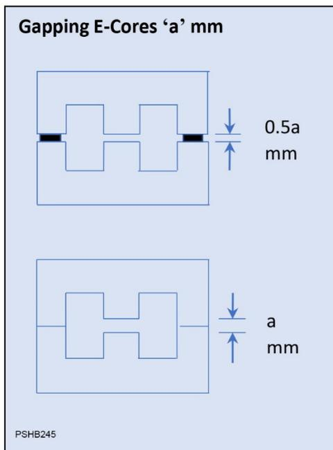
**Figure 7.6** Gapping E-cores
