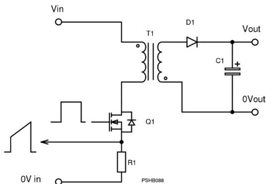
**Figure 7.12 Current mode control uses ramp from R1 for PWM**
