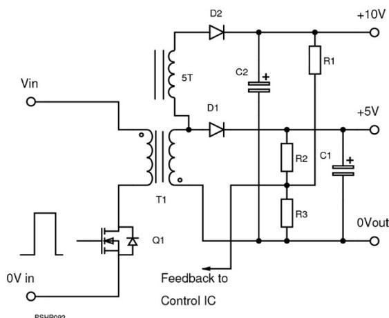
**Figure 7.15** Sharing regulation between multiple outputs
